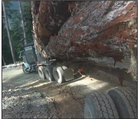
**Figure 4. A loaded 7-axle highway configuration logging truck navigates a steep switchback.**
