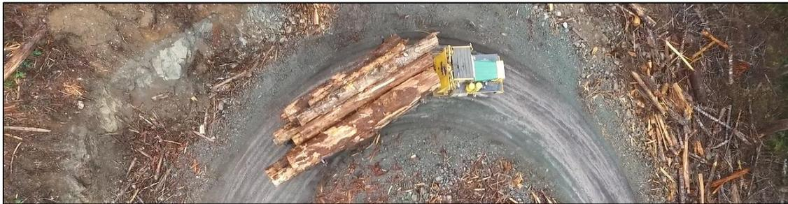
Figure 1. View from a UAV of a 5-axle off-highway truck negotiating a tight switchback.
