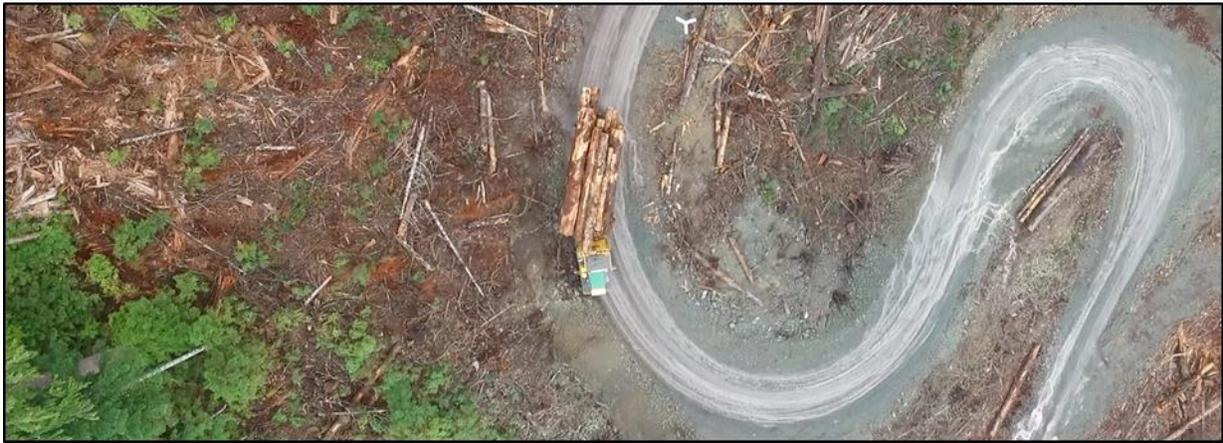
**Figure 3. View from the UAV of a 5-axle off-highway truck entering the first of two curves in Switchback #3.**
